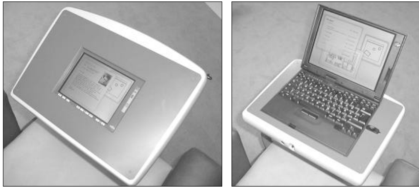
Fig. 6. left - CommChair with integrated pen-based computer, right - CommChair with docking facility for standard laptops.
